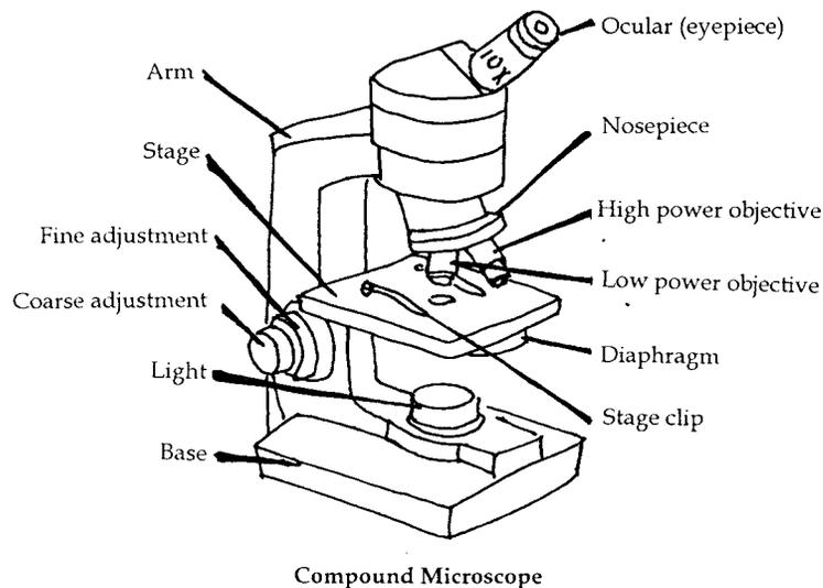
*Figure 1: Components of the Compound Microscope*
