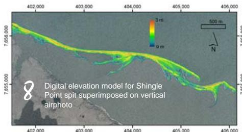
Digital elevation model for Shingle Point spit superimposed on vertical airphoto
