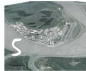
Flood extent (5) at Aklavik (5) during high spring flooding, as experienced 5 June 1992, simulated by flooding the LiDAR DEM, validated by RTK ground surveys and traditional knowledge.
