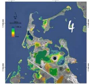
Flood extent (3) and flood depth (4) at Tuktoyaktuk, simulated by flooding the LiDAR DEM for a storm surge equivalent to the September 1993 event (2.51 m CD) with a projected sea-level rise of 0.31 m
