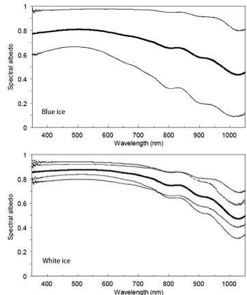
The figures show the extremes (thin lines) and averages (thick lines) for spectral albedo observed over blue ice and white ice surfaces between YD 97-121.
