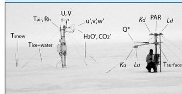
Continuous sampling at Button Bay field site from YD 78 (19 March) to 123 (3 May) in 2005. Parameters included air temperature, relative humidity, wind speed, wind direction, turbulent fluxes of heat, water vapour, momentum and  $CO_2$  in the atmospheric boundary layer, ice and snow temperatures using thermocouple strings extending through the ice/snow cover, surface skin temperature and the components of the surface radiation balance.
