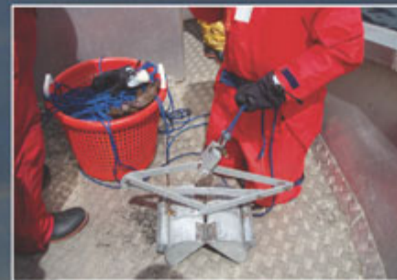
Figure 6. Mini-ponar grab sampler used to sample marine benthos.
