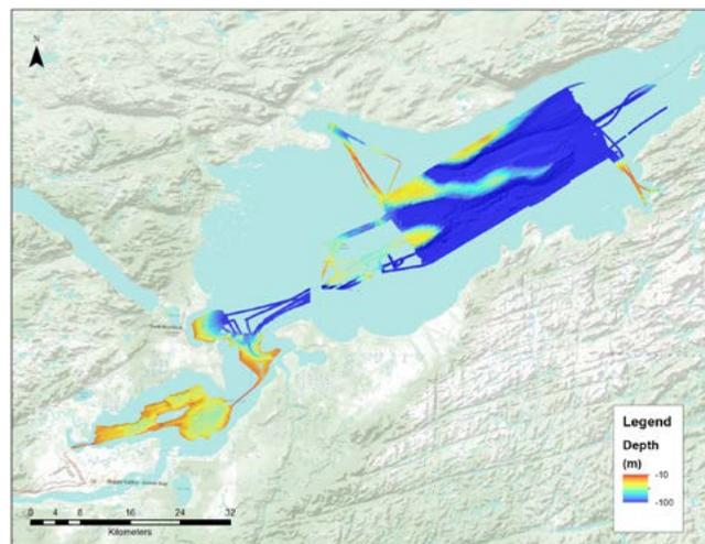
Figure 3. Multibeam sonar-derived bathymetry from Lake Melville collected in 2013
