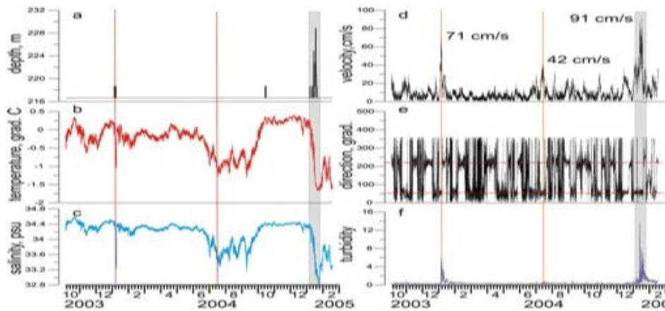
Figure 2. Time series of (a) pressure, (b) water temperature, (c) salinity, (d) velocity, (e) current direction and (f) turbidity from mooring CA13-03 at 216 m depth. Gray shading indicates shelf-break wind-forced current event in January 2005.
