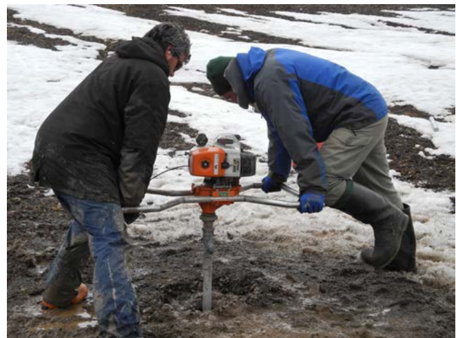
Figure 4. ADAPT permafrost drilling in support of the ArcticNet water track research on Ward Hunt Island. Photo: W.F. Vincent (CEN/ArcticNet).
