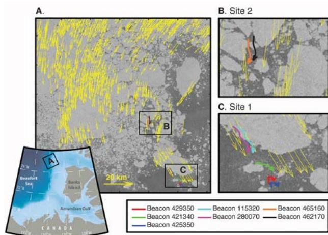
Figure 9. Radarsat derived ice motion between images acquired on Aug. 17, 15:17 and Aug. 18, 15:35, 2011 illustrating the average ice motion (yellow vectors). Beacon data are shown in other colours and in general show good agreement between the general ice motion and the motion of floes. This is particularly valid for first year ice floes (Komarov and Barber 2013; Barber et al. 2014).
