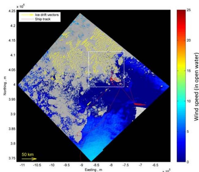
Figure 8. Ice drift and surface wind speed estimated from a model relating RADARSAT-2 backscatter to surface winds. RADARSAT-2 HH-HV Image acquired on Aug 16, 15:46, 2011 (Komarov et al. 2013; Barber et al. 2014).
