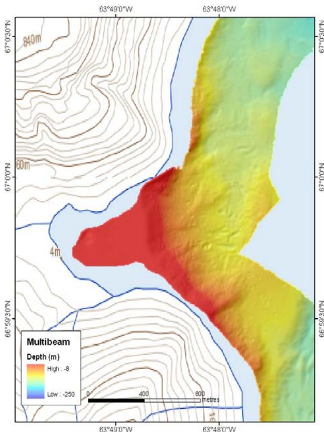
Figure 8. Colour shaded-relief bathymetry of submerged side-entry delta terrace at -18 m in Kangert Fiord, Cumberland Peninsula, south of Qikiqtarjuaraq, NU (see Figure 2 for location), acquired using the EM3002 multibeam sounder on MV Nulijuk, with assistance of UNB Ocean Mapping Group (project 2.6).
