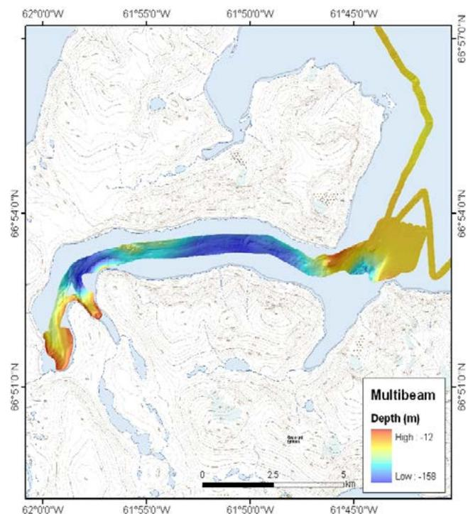
Figure 9. Colour shaded-relief bathymetry of -50 m terrace on sill of Akpait Fiord and small delta at same level in side entry valley near the head of the fiord (see Figure 2 for location). Data acquired as for Figure 8.
