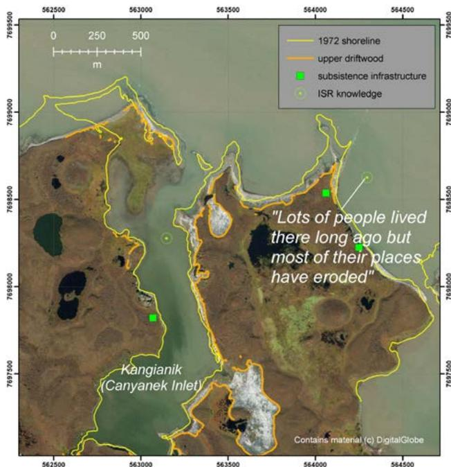
Figure 11. Subsistence infrastructure at Kangianik (Canyanek Inlet), south coast of Kugmallit Bay in the southern Beaufort Sea (see Figure 4 for location); shows 1972 shoreline vector superimposed on 2010 satellite image; also extreme water levels, as indicated by upper limits of driftwood; and example of georeferenced traditional knowledge from ILA records (source: Forbes et al., 2013).
