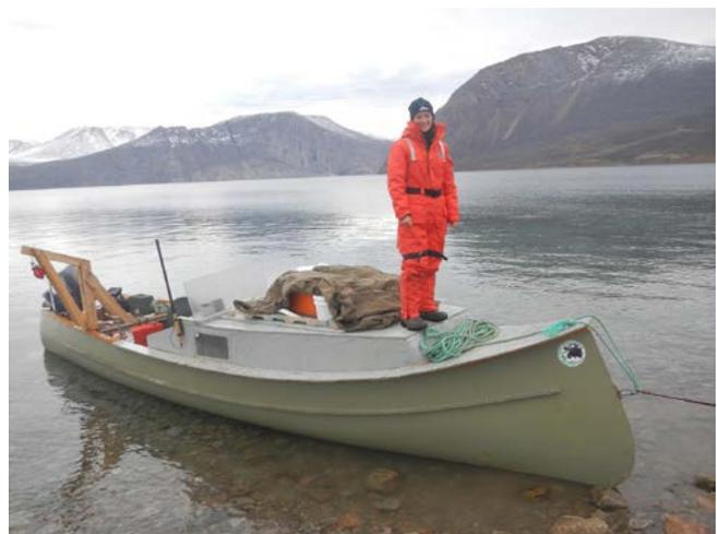
Figure 1. Survey vessel (locally chartered freighter canoe) used for coastal and benthic surveys in the vicinity of Qikiqtarjuaq (Broughton Island) in 2013. Research assistant Jenna Munden on the bow and Broughton Channel in background. Note sampling frame with block and single-beam sounder with transom-mounted transducer (photo credit: Beth Cowan).
