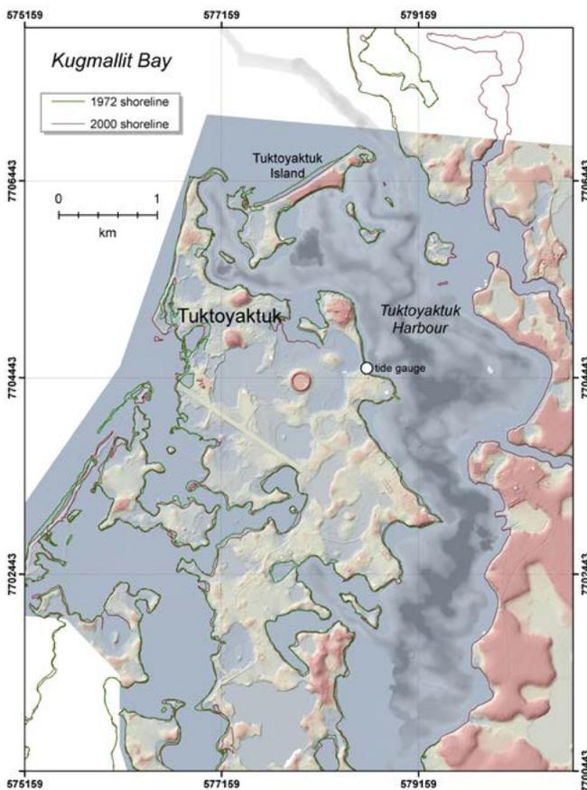
Figure 6. Colour-shaded relief topography (pink shades high), grey-scale multibeam bathymetry (in harbour), and sidescan sonar mosaic (seabed outside harbour) at Tuktoyaktuk, NWT (modified after Forbes et al., 2014b). Note 1972 and 2000 vector shorelines, showing rapid erosion along the outside of Tuktoyaktuk Island, extension of southwestern spit, and rapid overstepping along the coast to the southwest.
