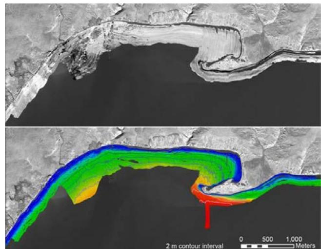
Figure 7. Bathymetry and sidescan backscatter image of Pauline Cove and Tethis Bay, Herschel Island, YT, acquired from small boat using interferometric sidescan sonar with real-time kinematic GPS positioning; onshore topography is grey-scale shaded-relief LiDAR image (Radosavljevic et al., 2013a, b).
