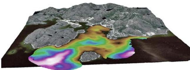
Figure 14. Oblique view of Hopedale in Nunatsiavut (NL), showing local topography, infrastructure and bathymetry, using WorldView satellite imagery draped over a digital elevation model.
